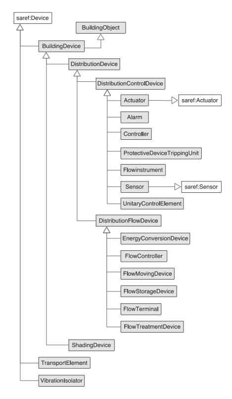
Figure 2: Device hierarchy in SAREF4BLDG (Part 1)
