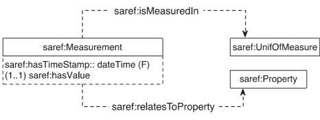
Figure 4: Measurement model
